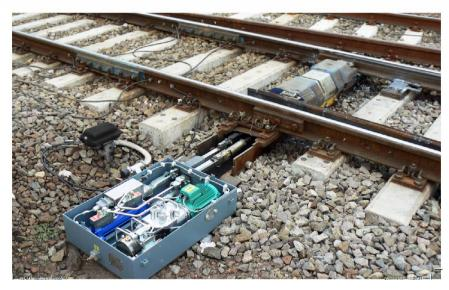
Upon new requirements of the users and of the application of new locking mechanisms, Műszer Automatika Kft has developed the outside driven Point Machine Family HVH-01-K. The new point machine is based on MA-HVH (01/D, 02) hydraulic point machines that have been manufactured for a several years already but it can be placed beside the points.
